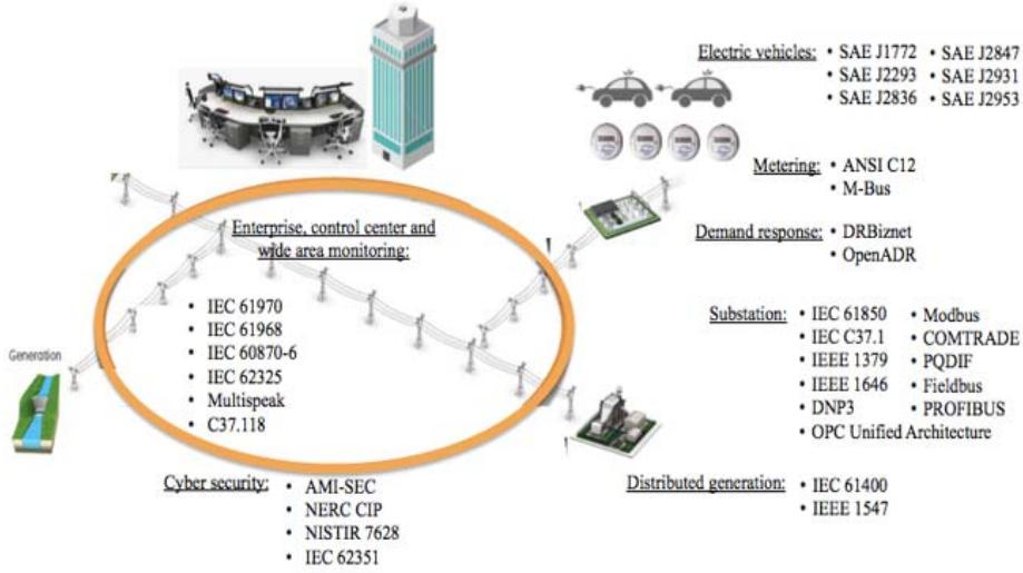
Figure 1. Commonly used smart grid standards and protocols
