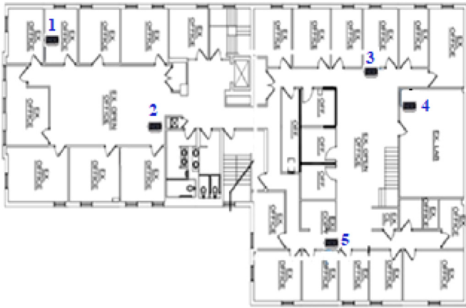
Fig. 1. Location of the five thermostats on the second floor within the building from which the compressors are controlled.
