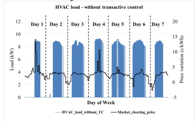
Figure 7. HVAC load profile without the transactive control
