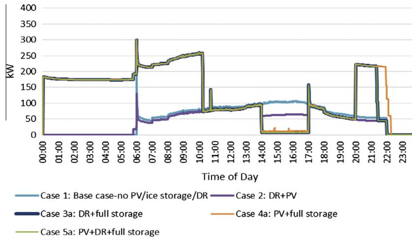
Fig. 11. Simulated building's HVAC power consumption profiles with combinations of PV, full ice storage and DR for the simulation day.
