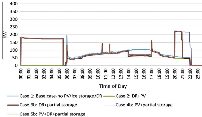
Fig. 13. Simulated building's HVAC power consumption profiles with and without PV, partial ice storage and DR for the simulation day.
