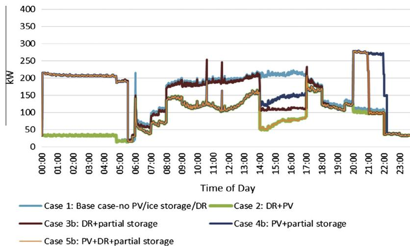
Fig. 12. Simulated building power consumption profiles with combinations of PV, partial ice storage and DR for the simulation day.
