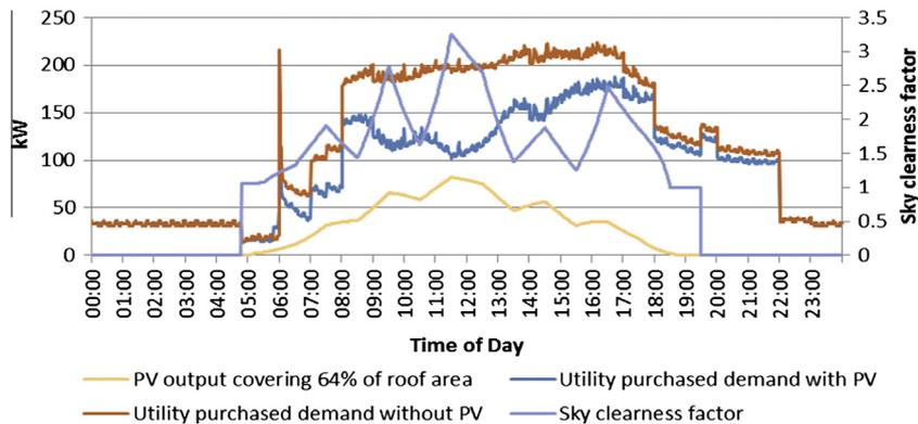
Fig. 4. Power generated by PV and purchased from utility for the simulated building for the simulation day.
