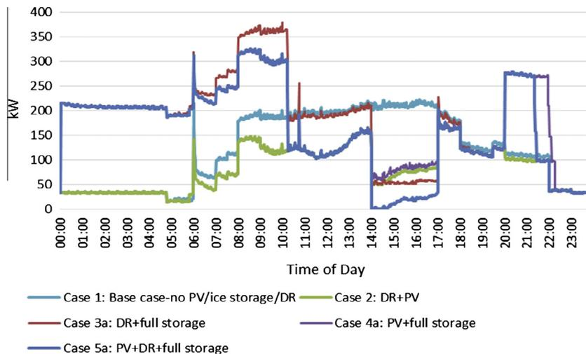
Fig. 9. Simulated building power consumption profiles with combinations of PV, full ice storage and DR for the simulation day.
