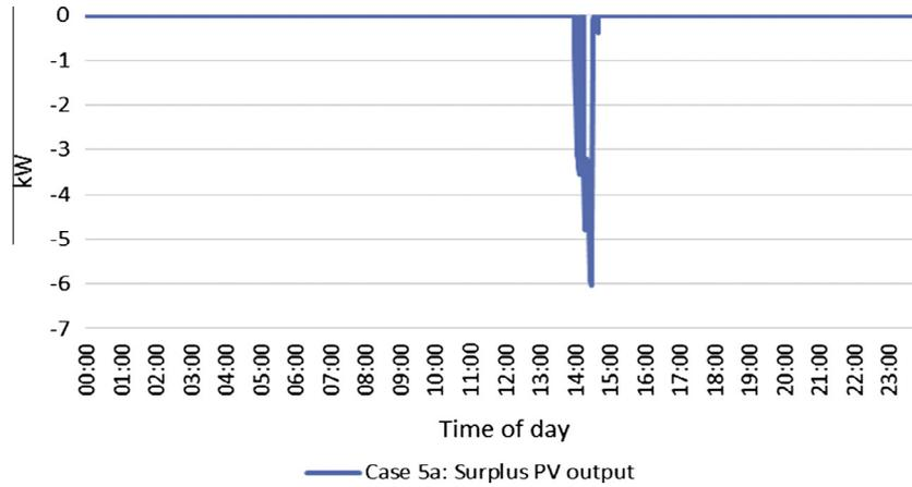
Fig. 10. Simulated building surplus PV power generation for Case 5a for the simulation day.
