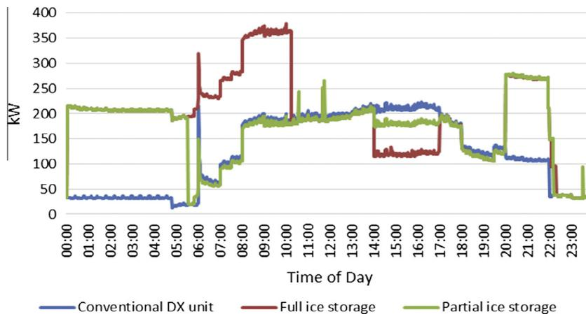
Fig. 5. Simulated building power consumption profiles with and without ice storage for the simulation day.
