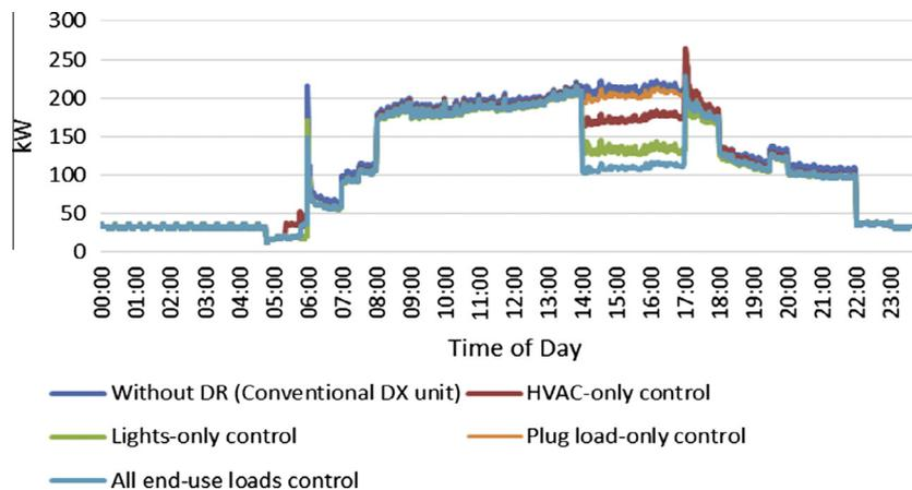
Fig. 7. Simulated building power consumption profiles with and without end-use loads control by EMS for the simulation day.
