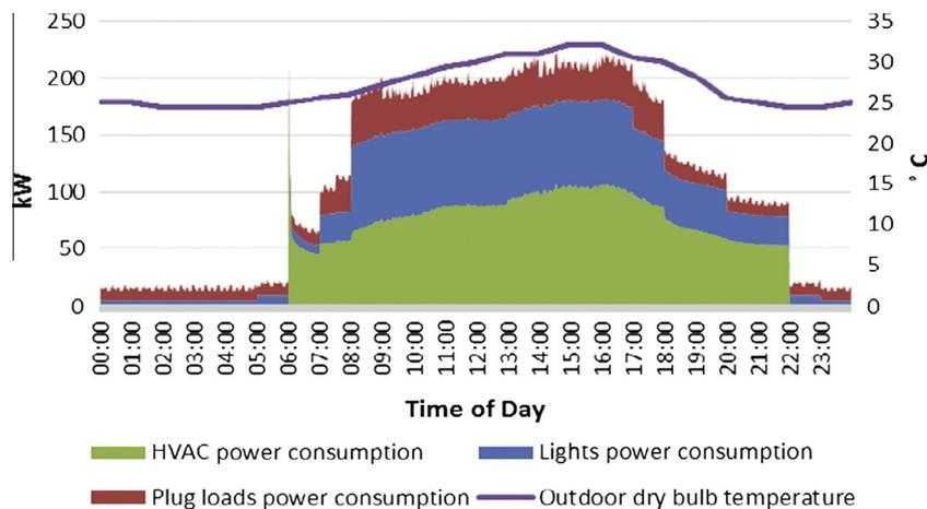
**Fig. 3.** Power consumption of major end-use loads for the simulated medium-sized office building for the simulation day.
