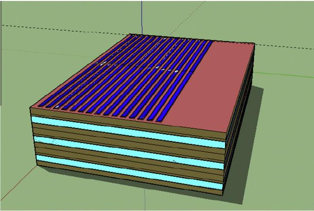
Fig. 1. Axonometric view of the simulated medium-sized office building with installed PV panels.
