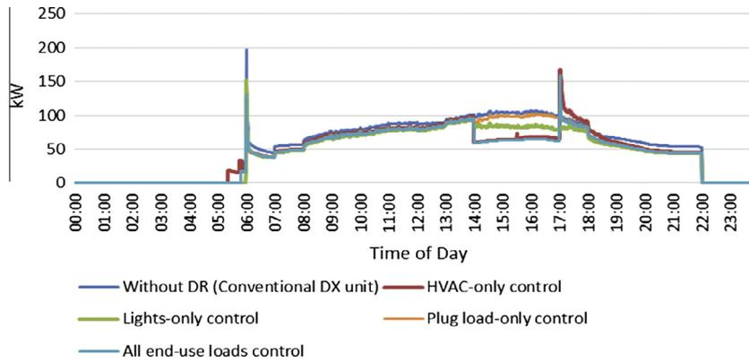
Fig. 8. Simulated building's HVAC power consumption profiles with and without end-use loads control by EMS for the simulation day.
