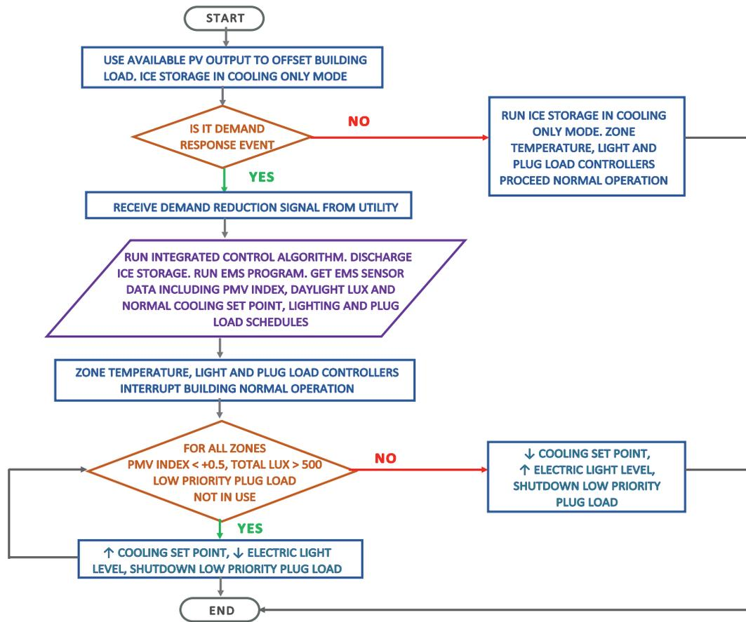
Fig. 2. Proposed integrated control model for building end-use loads, PV and ice storage.
