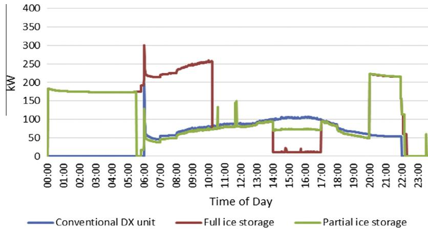
Fig. 6. Simulated building's HVAC power consumption profiles with and without ice storage for the simulation day.
