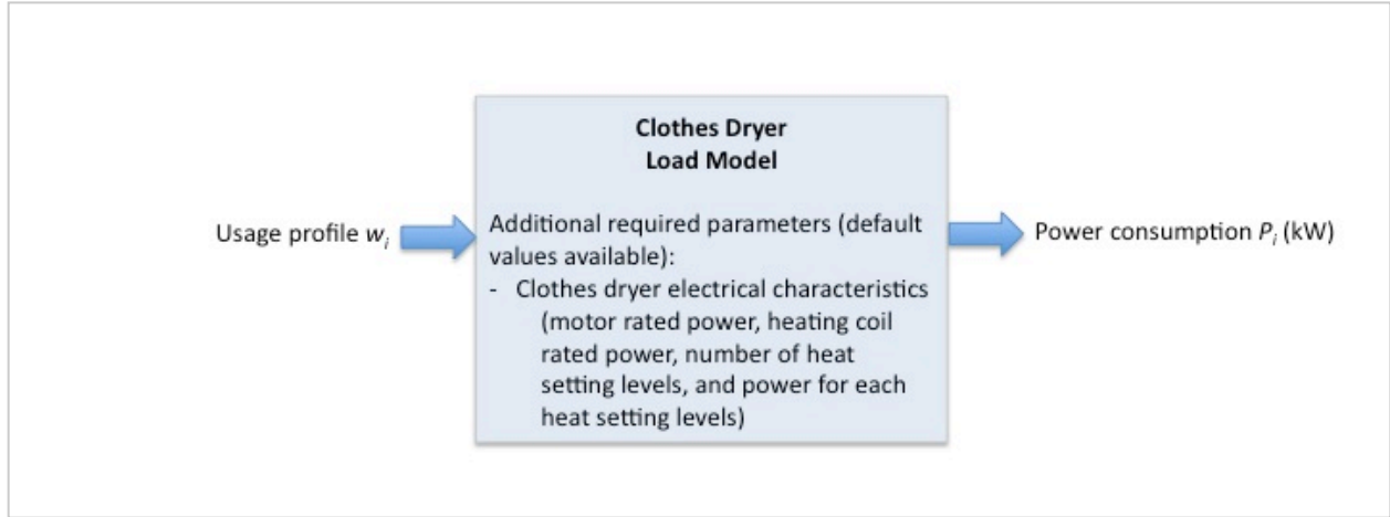
Fig. 4-22. Clothes dryer load model block diagram
