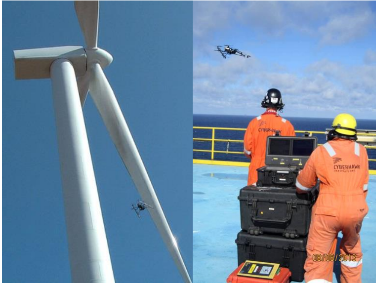
Piloted UAV inspection of land-based turbine (left) and offshore oil & gas platform (right)
